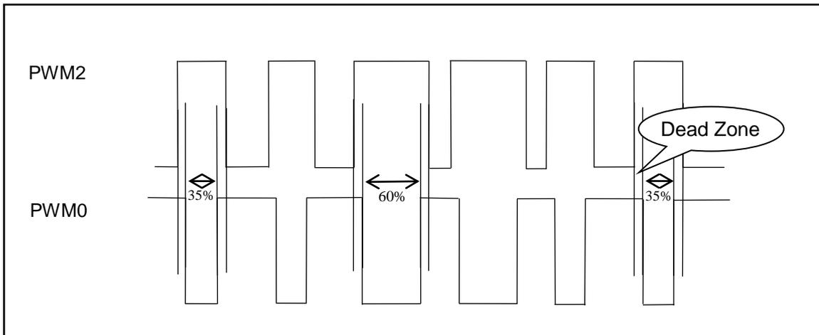
User can find that above example only provides dead zone where PWM are both in high. If need dead zone where PWM are both in low, you can realize it by resetting each control register's Inverse like:
