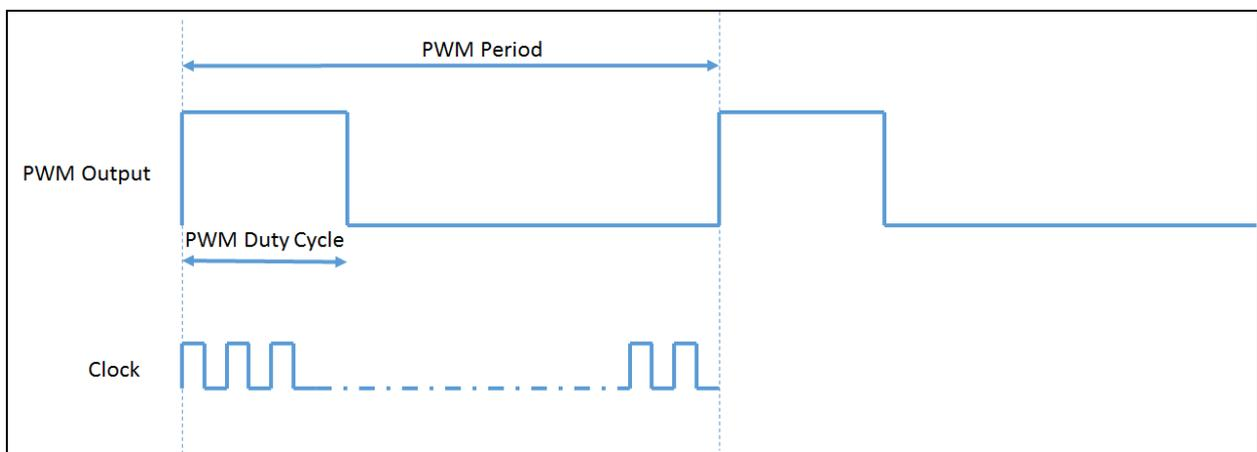
Fig.14: PWM Output Waveform
