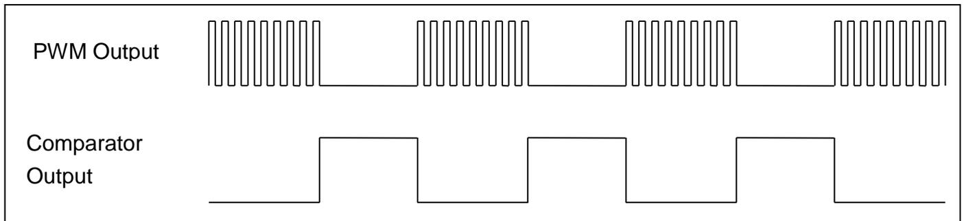
Fig.13 : Comparator controls the output of PWM waveform
