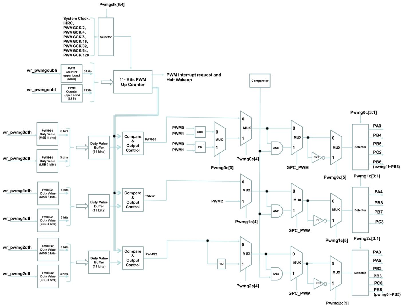
Fig.15: Hardware diagram of whole set of triple SuLED 11-bit PWM generators
