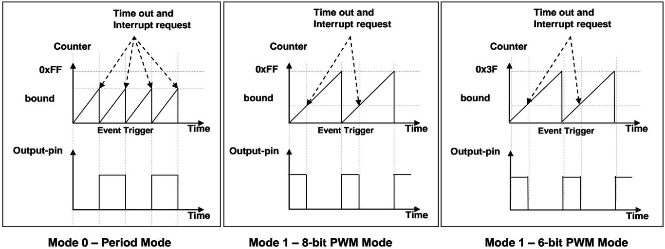
Fig.12: Timing diagram of Timer2 in period mode and PWM mode (tm2c.1=1)
