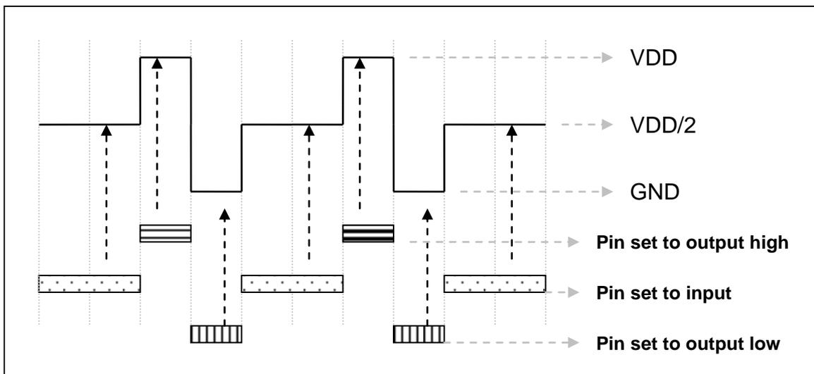
Fig. 9: Using VDD/2 LCD bias voltage generator
