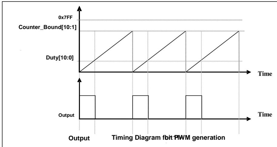
Fig.16: Output Timing Diagram of 11-bit PWM Generator
