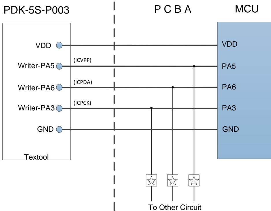
The above figure shows the connection for PFS123 on-board writing. In this figure, ☆ can be either resistors or capacitors. They are used to isolate the programming signal wires from the peripheral circuit. it should be  $\geq 10K\Omega$  for resistance while  $\leq 220pF$  for capacitance.
