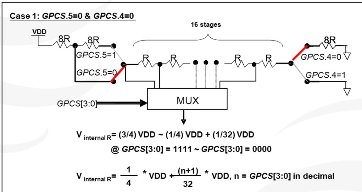
Fig. 31:  $V_{\text{internal R}}$  hardware connection if  $GPCS.5=0$  and  $GPCS.4=0$
