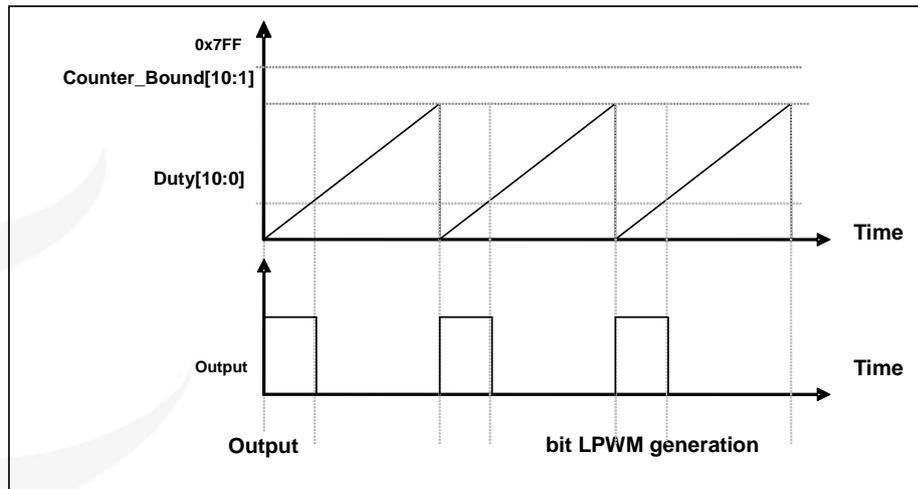
Fig. 26: Output Timing Diagram of 11-bit LPWM Generator
