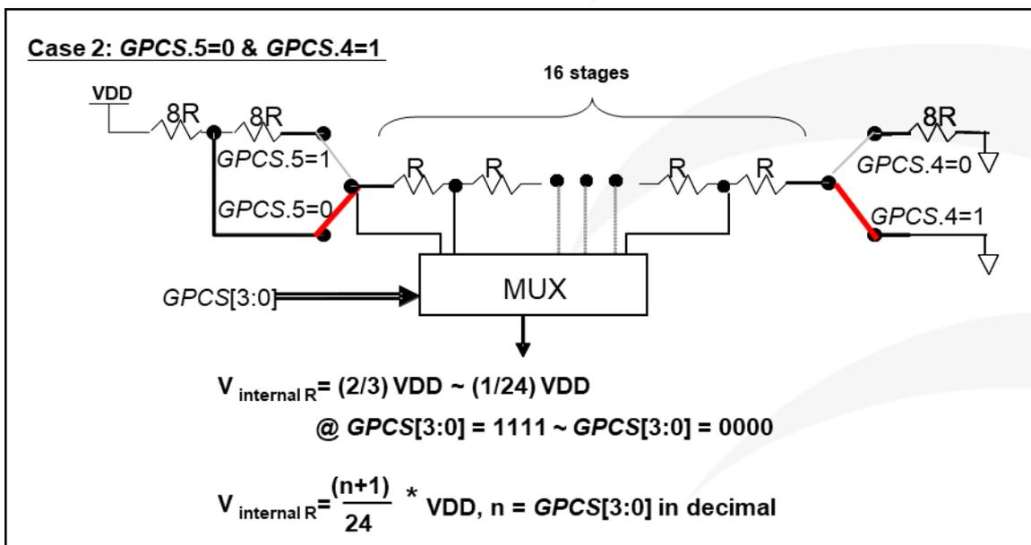
Fig. 32:  $V_{\text{internal R}}$  hardware connection if  $GPCS.5=0$  and  $GPCS.4=1$
