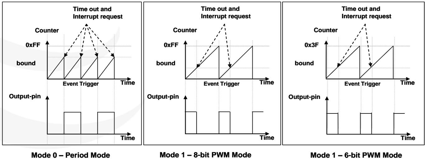
Fig. 19: Timing diagram of Timer2 in period mode and PWM mode ( $TM2C.1=1$ )
