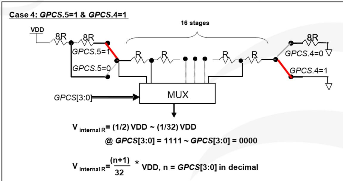
Fig. 34:  $V_{\text{internal R}}$  hardware connection if  $GPCS.5=1$  and  $GPCS.4=1$
