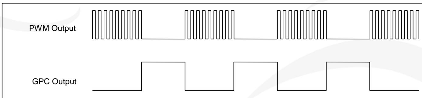
Fig .30: Comparator results control PWM output
