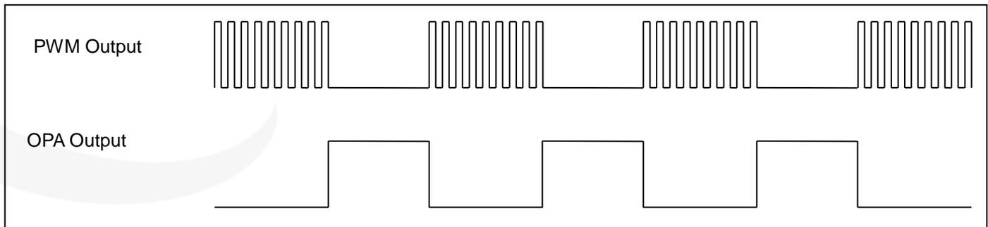
Fig. 37: OPA comparator mode control PWM output
