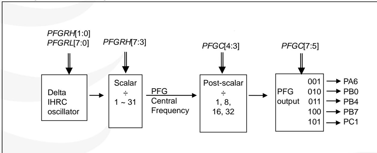
Fig. 43: Hardware Diagram of PFG
