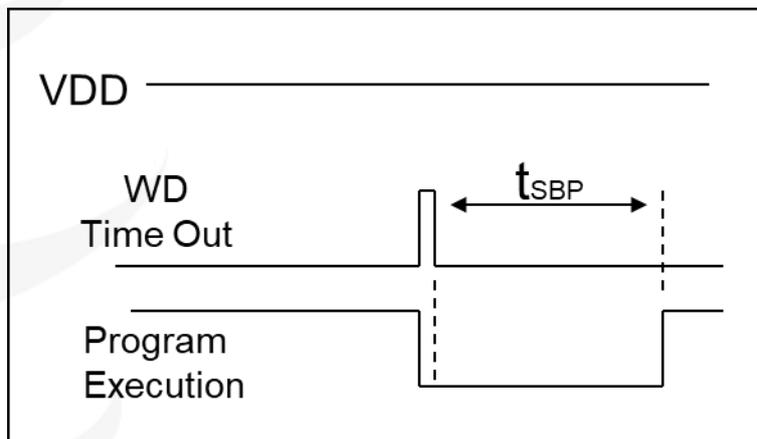
Fig. 13: Sequence of Watch Dog Timeout reset
