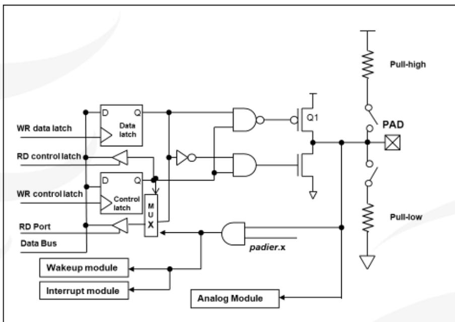
Fig. 16: Hardware diagram of IO buffer
