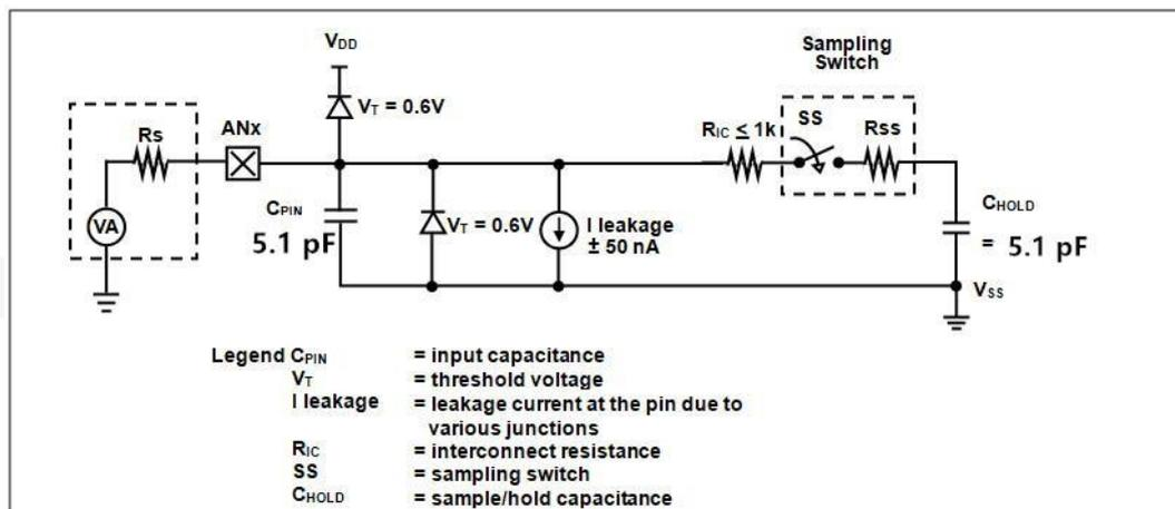
Fig.39: Analog Input Model
