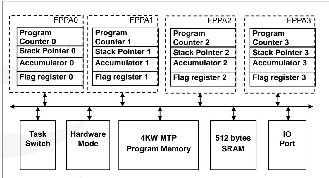
Fig. 1: Hardware Diagram of FPPA units
