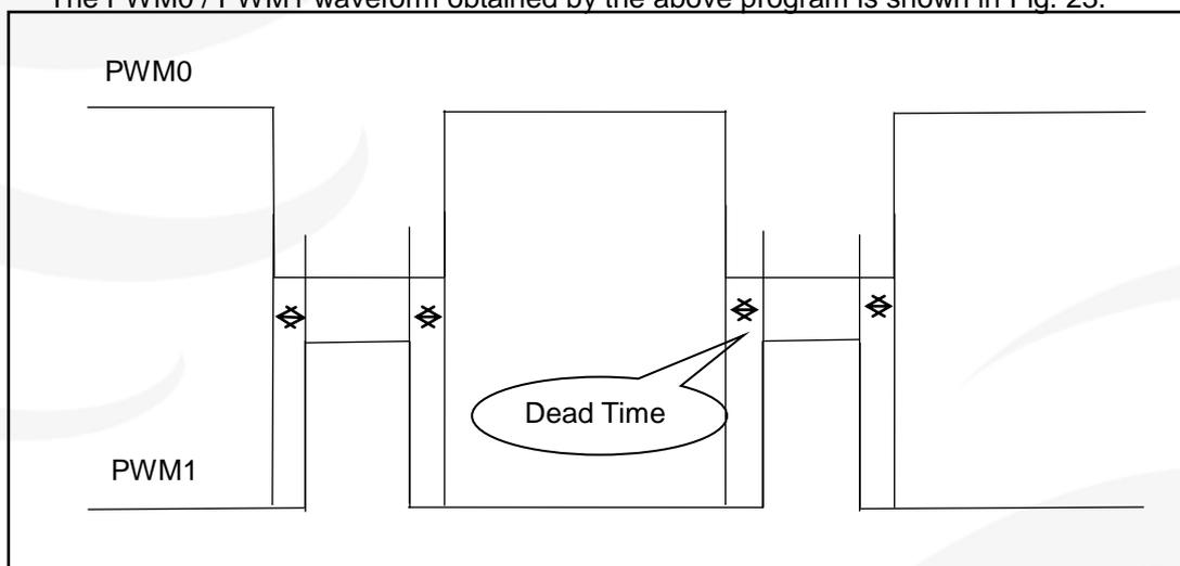
Fig. 23: Two complementary PWM waveforms with dead zones
