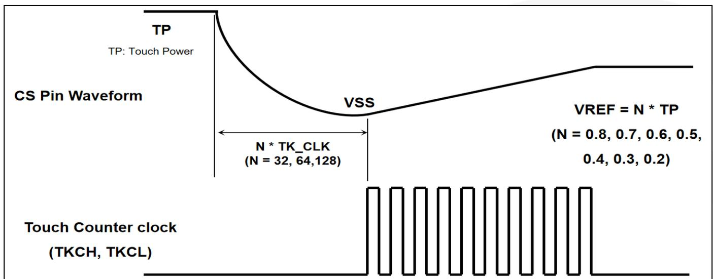
Fig. 42: Timing diagram of Touch converting progress
