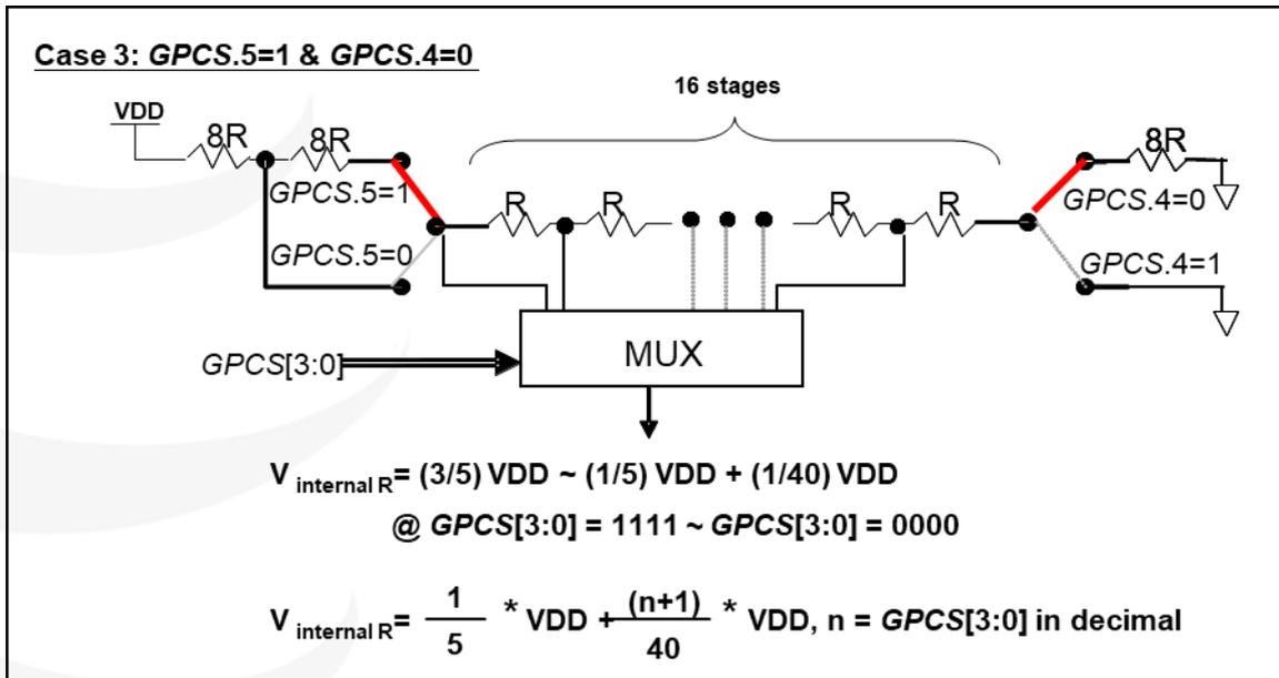
Fig. 33:  $V_{\text{internal R}}$  hardware connection if  $GPCS.5=1$  and  $GPCS.4=0$
