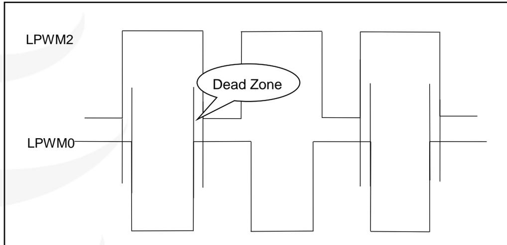
Fig.27: Complementary LPWM waveform with dead zones
