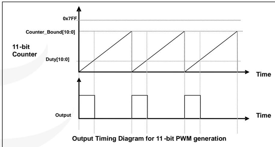
Fig. 22: Output Timing Diagram of 11-bit PWM Generator
