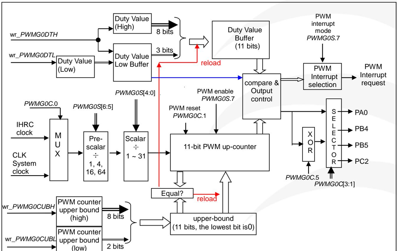
Fig. 21: Hardware Diagram of 11-bit PWM Generator 0 (PWMG0)
