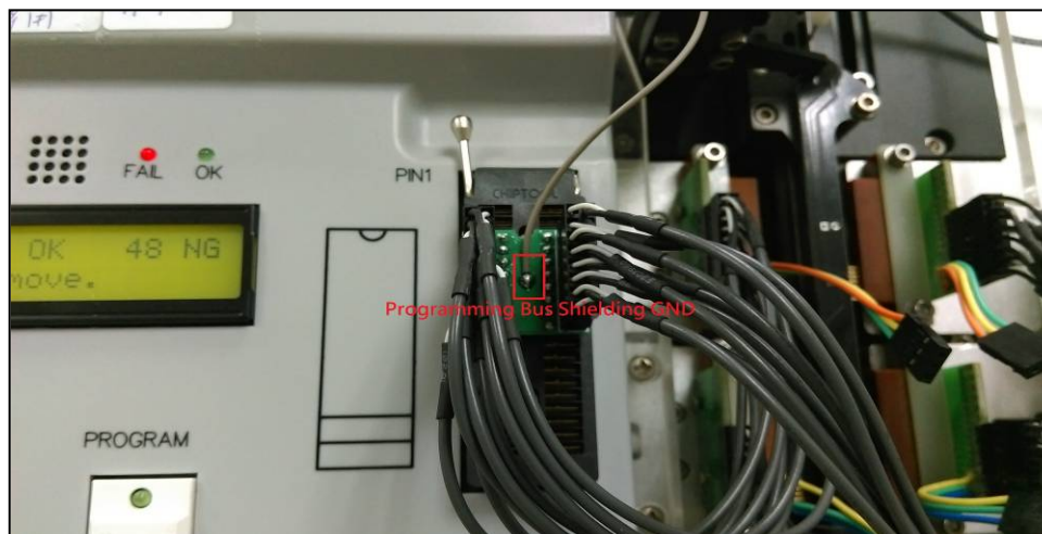
Fig. 5 : The outlet terminal of the writing bus wires and the shielded ground line
