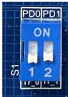
Fig. 9: Communication Enable Section
