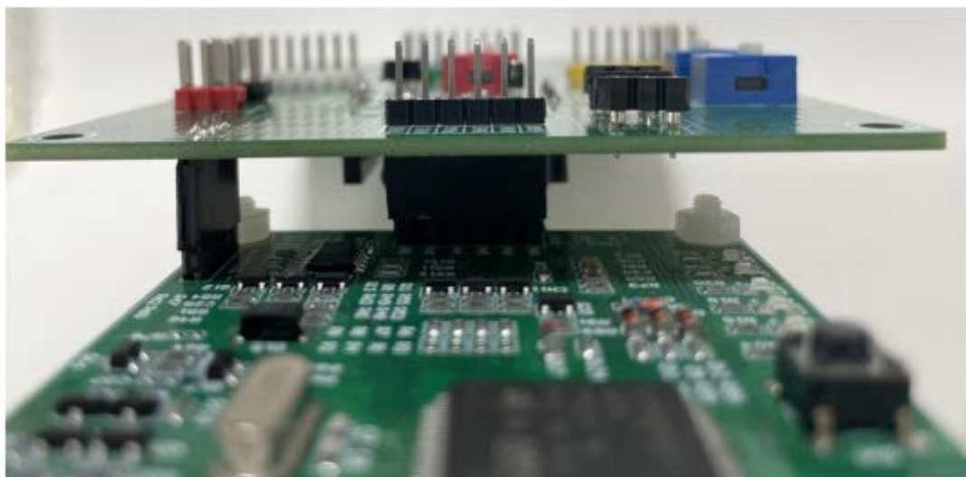
Fig. 18: Side of connection between 6S-EMB and 5S-P-C01
