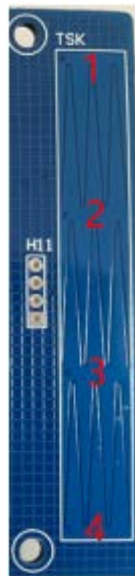
Fig. 13: Touch Control Slider Section
